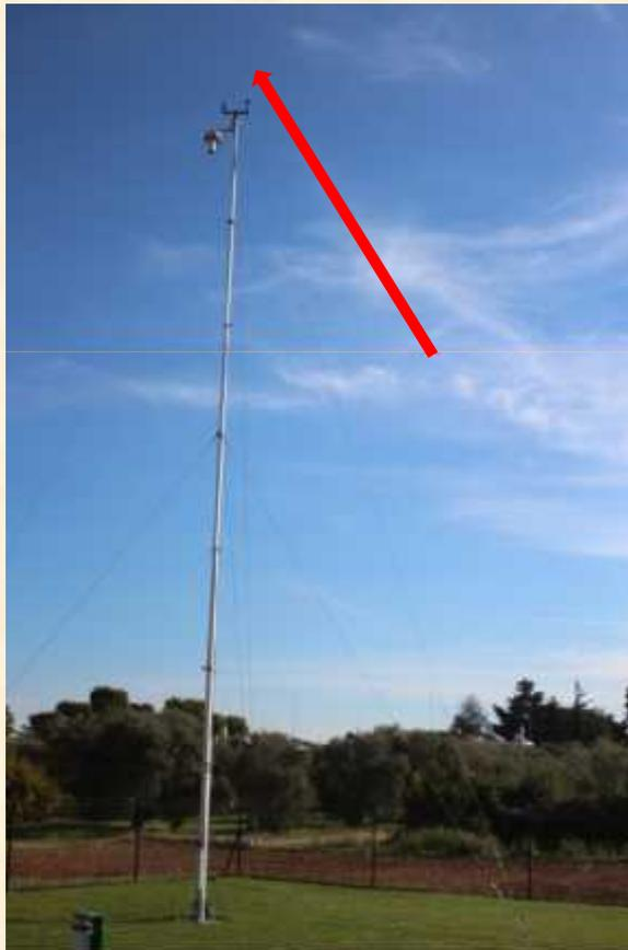
Anemometer at 10 meters
